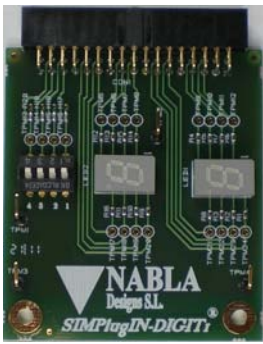
SIMPlugIN-DIGIT - 2 hex digit displays - 4 switches - 20 test-points
