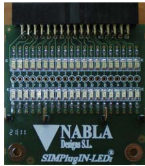
SIMPlugIN-LED - 20 red leds (when 0 logic level) - 20 green leds (when 1 logic level) - 20 test-points
