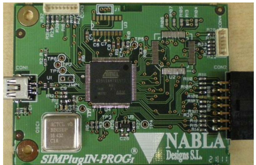
SIMPlugIN-PROGRAMMER - JTAG programming - SPI programming - simple USB interface (software included with the board)
