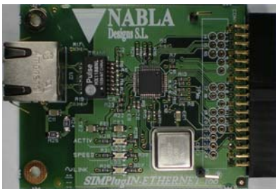
SIMPlugIN-ETHER100 - Ethernet 100Mbit / 10 Mbit - test-points for all relevant signals
