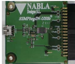
SIMPlugIN-USB - USB full speed (12 Mbit) USB 2.0 - test-points for all relevant signals
