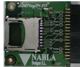
SIMPlugIN-SD - SD card slot - test-points for all relevant signals
