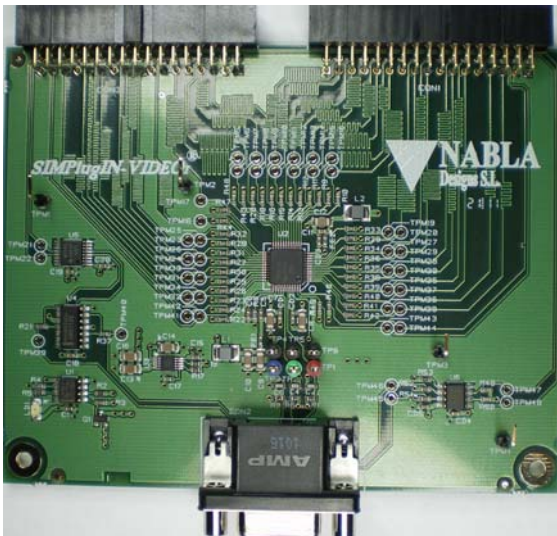
SIMPlugIN-VIDEO - high speed, 10 bit, triple video DAC - complete VGA port - also composite video - also general purpose triple DAC - test points for all relevant signals
