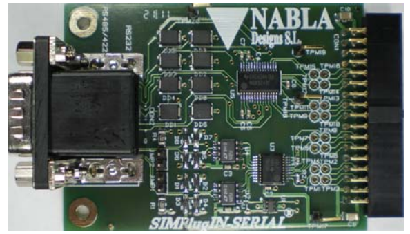
SIMPlugIN-SERIAL - 1 complete RS232 port - 2 RS485 ports (or 1 RS422 port) - simultaneous operation of all ports - Testpoints for all relevant signals
