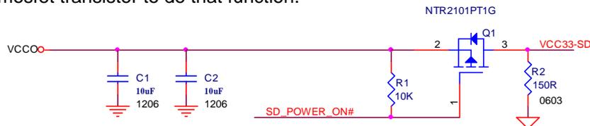
When the signal SD\_POWER\_ON# is active (low) the mosfet transistor is on and the SD card is powered. When the transistor is off and the SD card is not powered and the resistor R2 acts as a small load that makes sure that VCC33-SD voltage reaches 0 volt in a reasonable time.
